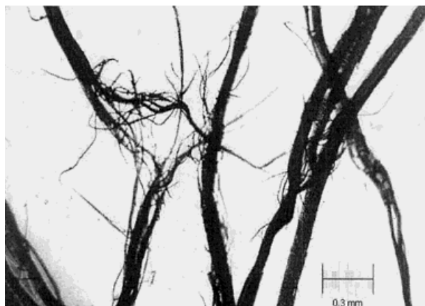
Figure 1 Micrograph of alkali-treated rice straws (magnification \times 100 ).
